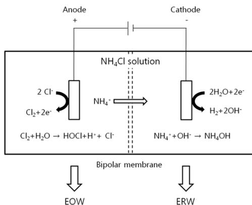
[Fig. 1] The principle of electrolysis of water.
