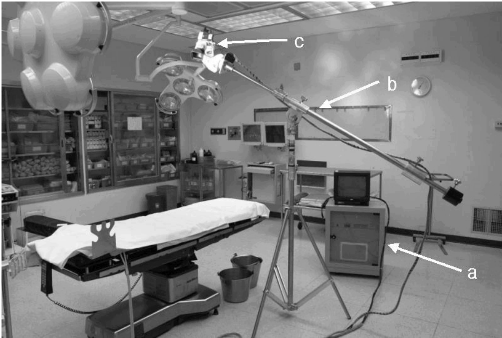
Fig. 1. Setting of equipments in the operating room for the tele-video education system. (a) control box: monitor, remote controller, video recorder, speaker, microphone (b) pan-tilt system (c) video camera
